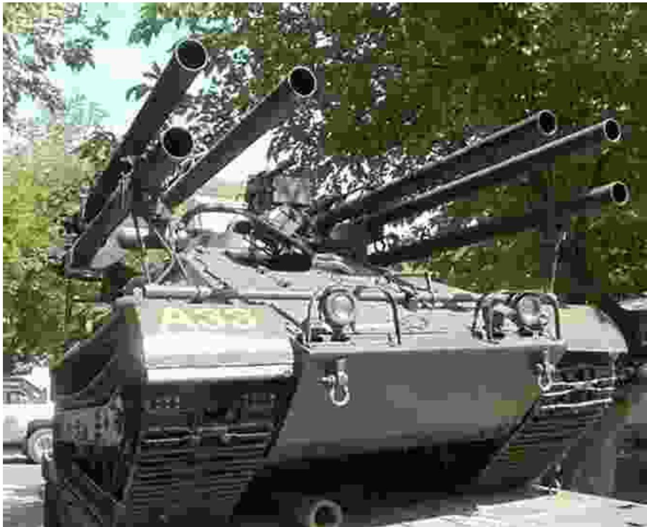
The M50 Ontos, a unique and compact anti-tank vehicle, complemented the Patton in the Marine Corps arsenal. Boasting six recoilless rifles, the Ontos could unleash a devastating barrage of high-velocity projectiles. Its small size and maneuverability allowed it to swiftly engage enemy armor in close quarters.
